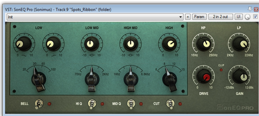
Here you can see the Sonimus SonEQ Pro settings Mike used to prepare the ribbon close-mics bus for mixdown: a combination of super-smooth high-frequency boost, to compensate for the mics' innate high-frequency roll-off, and high-pass filtering, to remove unwanted spill from the PA system of a dance party that unexpectedly kicked off in the neighbourhood just as takes were beginning!
